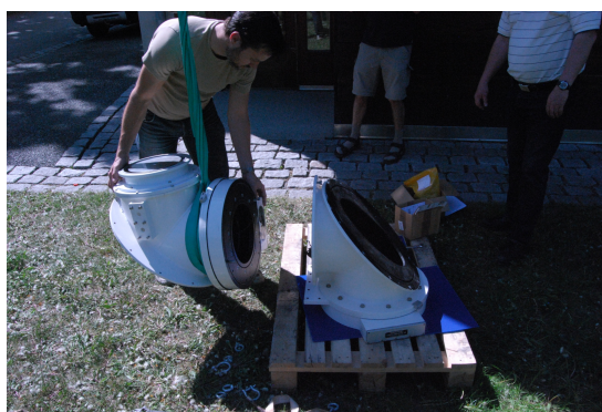
Figure 17: Mirror gluing and turret assembly prior to mounting
