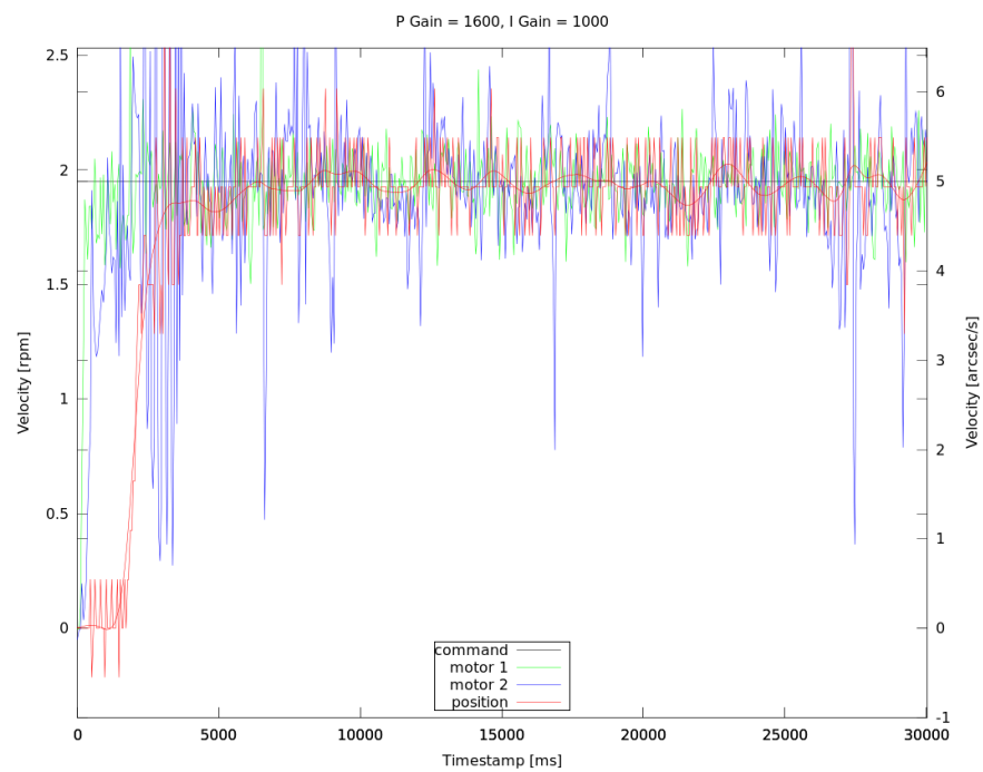
Figure 13: Well chosen parameters (P=1600, I=1000)
