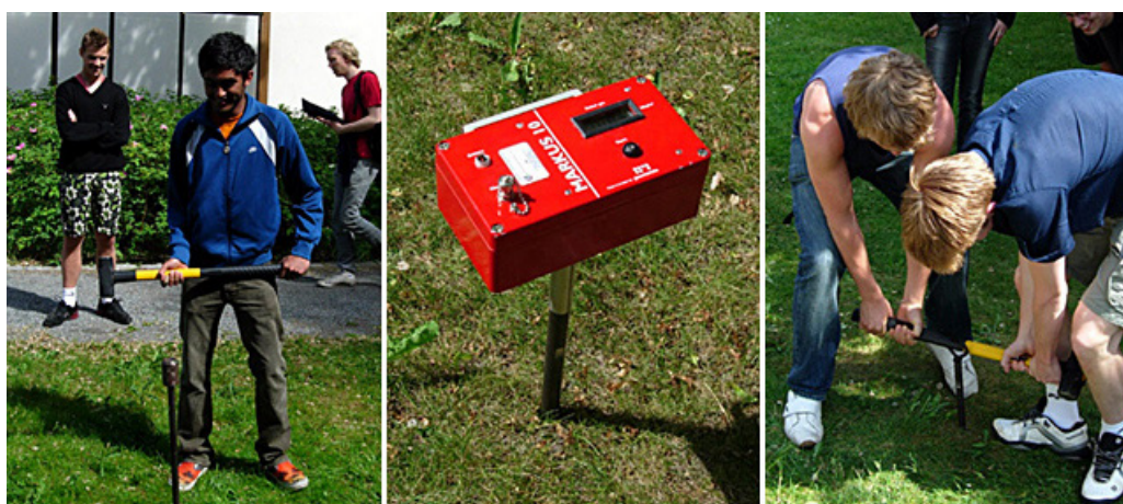
Figure 8. Measurements of radon content in ground air with the Markus instrument during the Summer Research School 2006.
