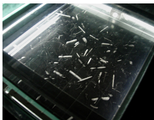
Figure 2. A photograph of the 40 \times 40 \text{ cm}^2 cloud chamber showing ionizing radiation including the thicker tracks from \alpha particles emitted in the decay of the radon and polonium nuclei. The radon content in the room was measured to be around 1600 \text{ Bq m}^{-3} . A short video sequence of the cloud chamber can be found in the online version of the journal at stacks.iop.org/physed/42/281 and [7].
