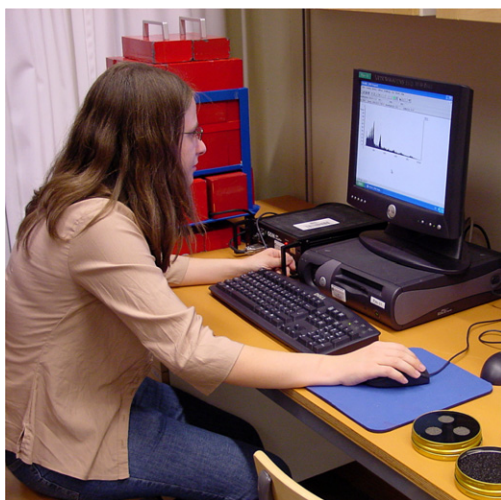
Figure 5. A student determining the radon content in air by measuring the \gamma radiation from ^{214}\text{Pb} from a coal container that has been exposed to air and radon gas over three days.
