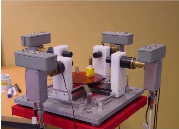
**Fig. 2 A simple PET camera. Each pair of movable detectors is coupled in coincidence. During the demonstrations the source is covered.**
